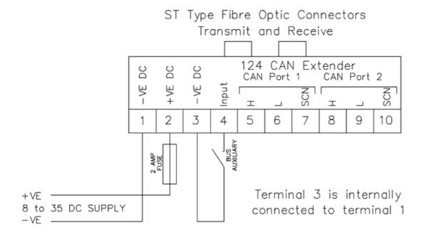
Bus auxiliary contact (terminal 4) is only required where a bus tie breaker is fitted.
