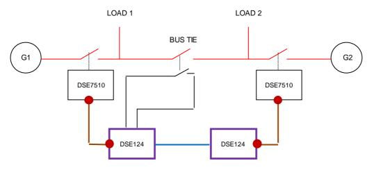
2 x MSC copper cable. Max 250m each 1 x fibre cable. Max 2km
